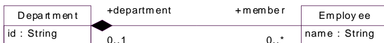
Figure 9.6 - Composite property serialized as XML elements, the opposite property is not serialized.
