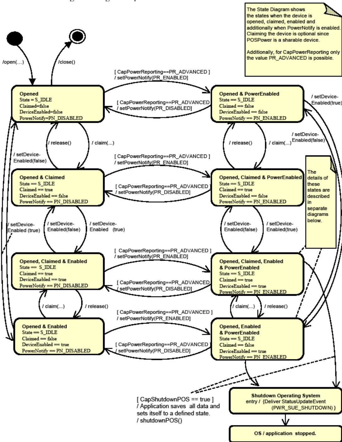
Fig. Chap. 29-4 Power State Diagram (POSPoer Control Device Model) POSPower PowerState Diagram - Part 1
