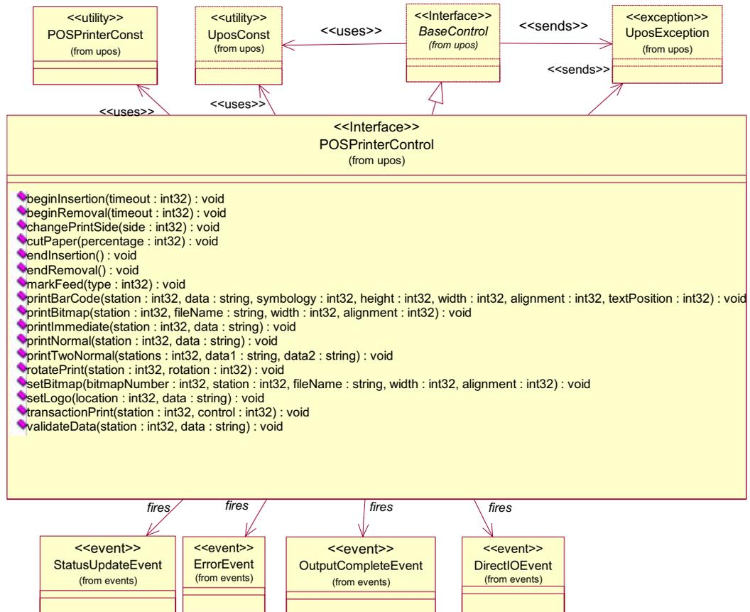
Only the methods of the POSPrinterControl are shown in order to avoid cluttering the diagram.
