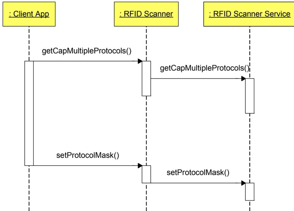
The following diagram shows a typical usage of a RFID Scanner device reading tags.
