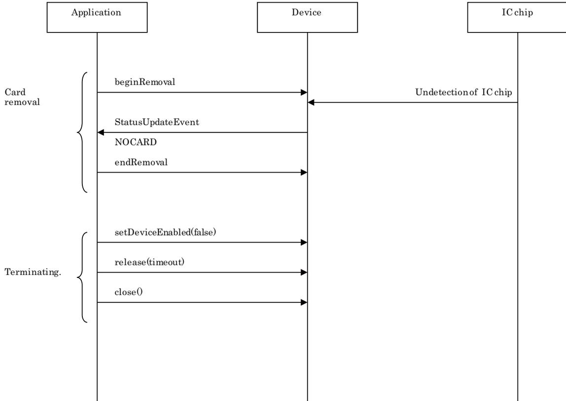
The following sequence diagram shows the CAT(EMV) usage that is used as EVR/W device. *Updated in Release 1.15*
