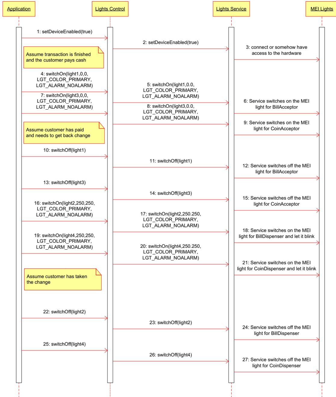
The following sequence diagram show the typical usage of the Lights device illustrating the handling of the pole lights.
