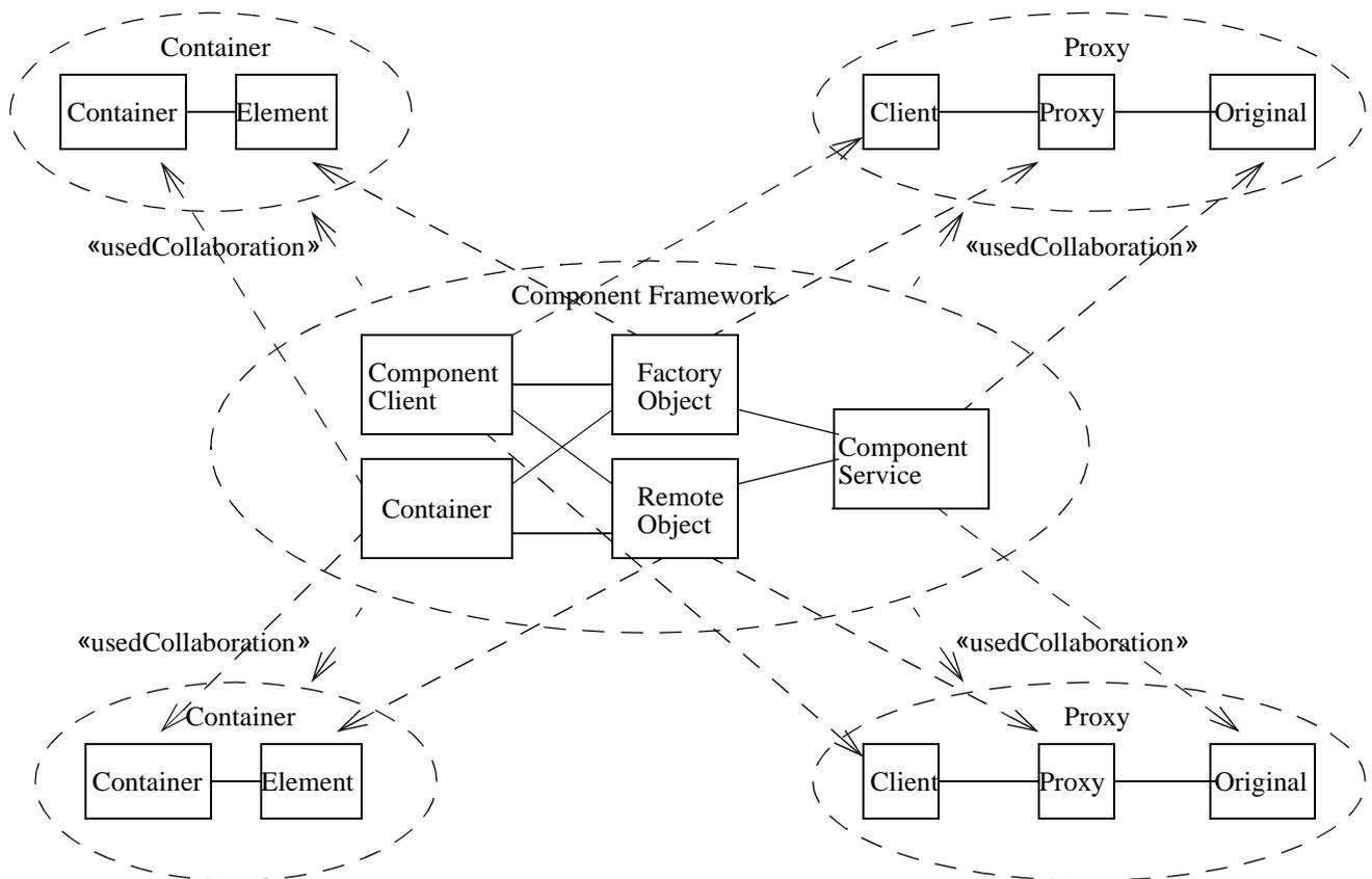
**Figure 99 - The ComponentFramework Collaboration uses two occurrences of the Proxy Collaboration and two occurrences of the Container Collaboration. Note that each role in the Component Framework corresponds to a role in two of the used Collaborations.**
