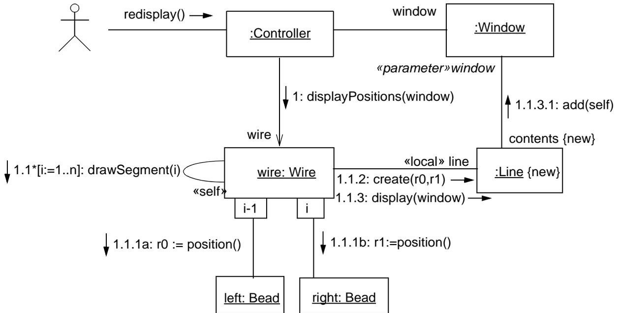
Figure 92 - Collaboration Diagram at instance level, presenting Objects, Links, and Stimuli referenced by a CollaborationInstanceSet and its InteractionInstanceSet.
