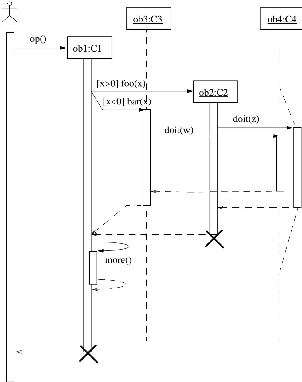
Figure 89 - Sequence Diagram with Focus of Control, Conditional, Recursion, Creation, and Destruction.
