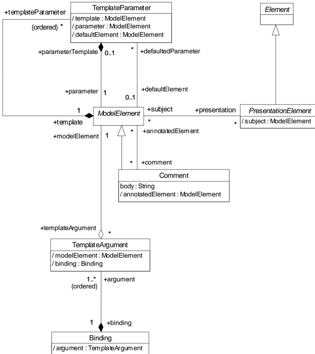
Figure 141 - Core Package - Auxiliary Elements
