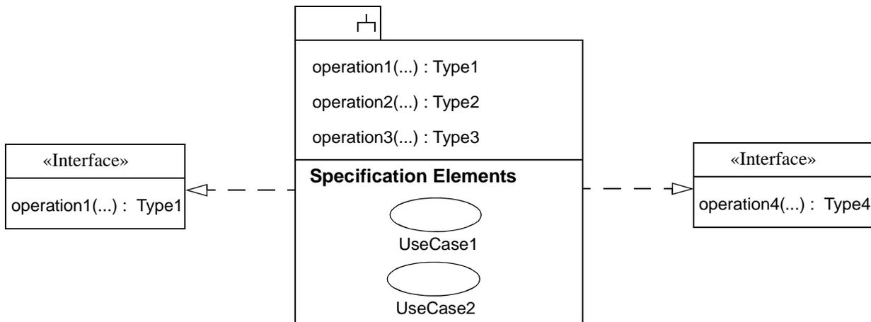
**Figure 45 - The specification part of a subsystem; compartment for realization part is suppressed. Implicit from the diagram is that the operation4(...) is either an operation of a specification element (UseCase1 or UseCase2) or of the subsystem itself. Furthermore, in cases where operations are used for the specification but only contained specification elements, there is no operations compartment, and vice versa.**
