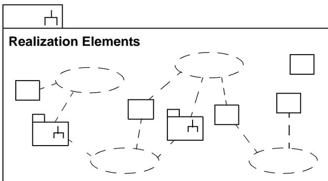
**Figure 46 - The realization part of a subsystem; compartments for specification part; that is, operations and specification elements are suppressed. Alternatively, collaborations could be shown in a separate diagram.**
