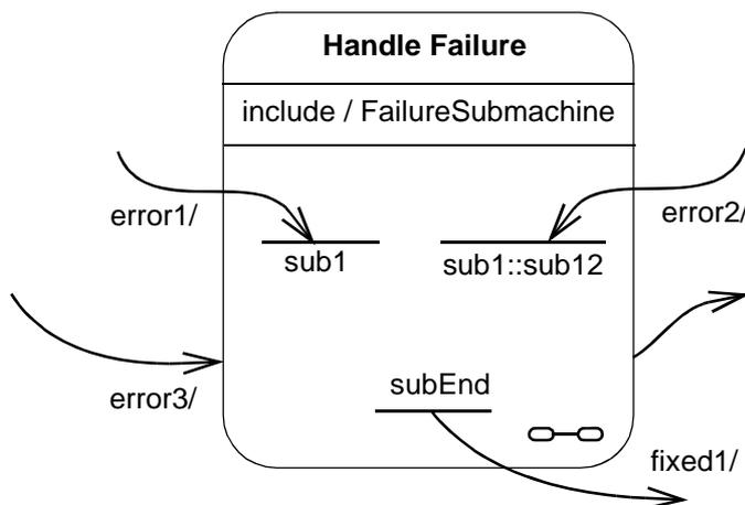
**Figure 115 - Submachine State**
