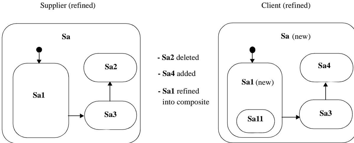
**Figure 29 - State Machine Refinement Example**
