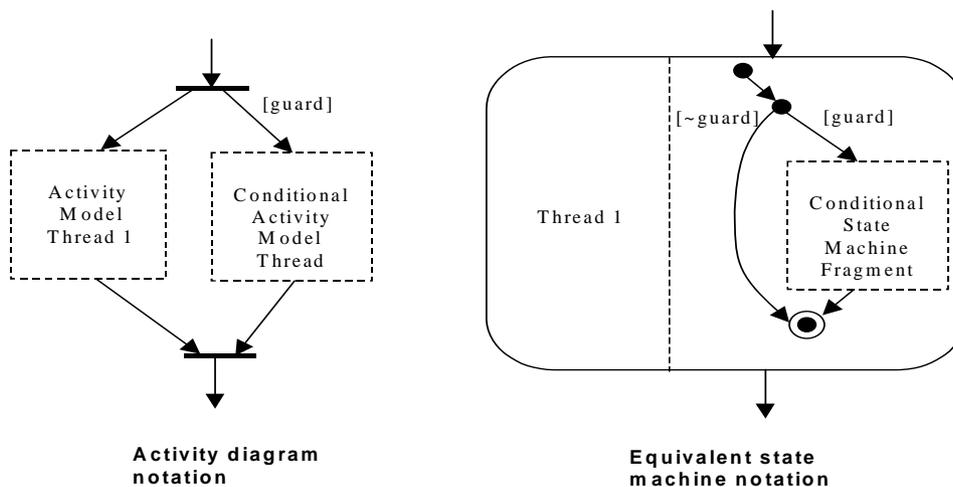
**Figure 31 - State machine meaning for an activity graph**
