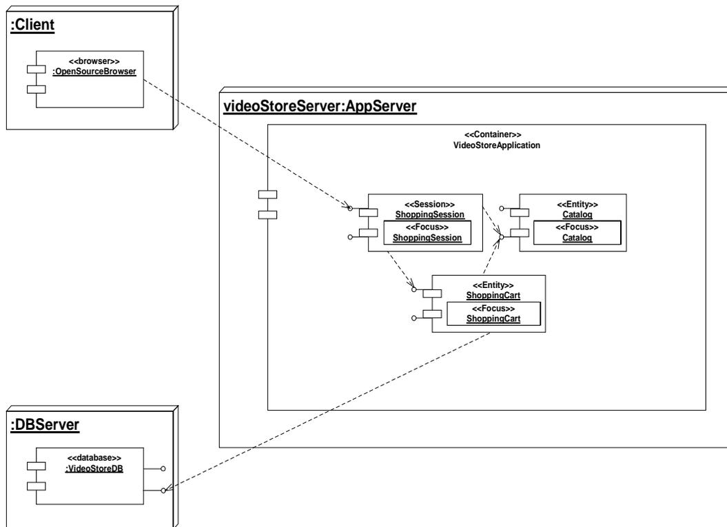
Figure 129 - Deployment Diagram
