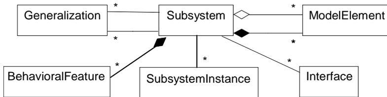
**Figure 34 - Subsystem illustration - shows Subsystem and its environment in the metamodel by flattening the inheritance hierarchy.**
