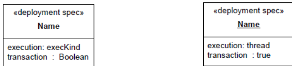
Figure 19.5 DeploymentSpecification for an artifact. On the left, a type-level specification, and on the right, an instance-level specification.
