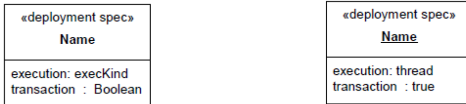
Figure 19.5 DeploymentSpecification for an artifact. On the left, a type-level specification, and on the right, an instance-level specification.
