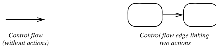
Figure 12.70 - Control flow notation
