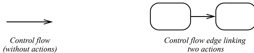
Figure 12.70 - Control flow notation
