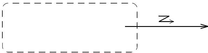
Figure 12.99 - InterruptibleActivityRegion notation with interrupting edge
