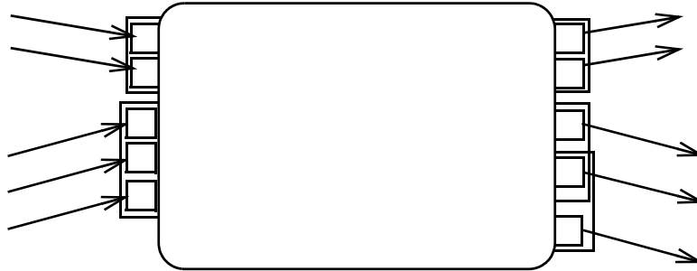
Figure 12.117 - Alternative input/outputs using parameter sets notation
