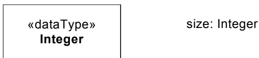
Figure 11.19 - Notation of data type: to the left is an icon denoting a data type and to the right is a reference to a data type that is used in an attribute.
