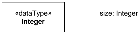
Figure 7.36 - Notation of data type: to the left is an icon denoting a data type and to the right is a reference to a data type that is used in an attribute.
