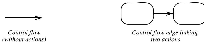
Figure 12.70 - Control flow notation
