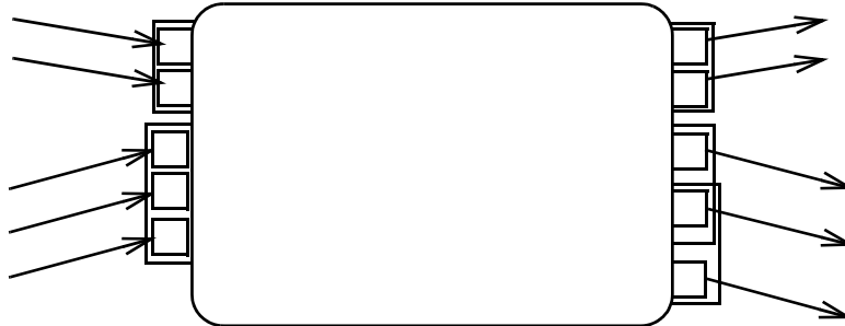
Figure 12.117 - Alternative input/outputs using parameter sets notation
