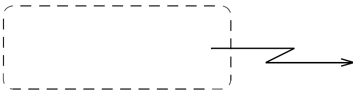
Figure 12.98 - InterruptibleActivityRegion notation with interrupting edge
