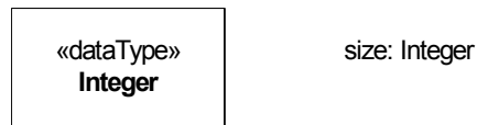
Figure 87 - Notation of data type: to the left is an icon denoting a data type and to the right is a reference to a data type which is used in an attribute
