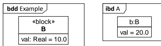
Figure 27: Default values and initial value in SysML
