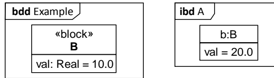
Figure 27: Default values and initial value in SysML
