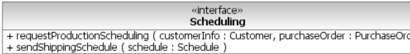
Figure 87: The Scheduling Service Interface
