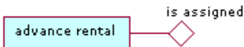
Figure H.9- Depicting the characteristic 'advance rental is assigned' using association notation
