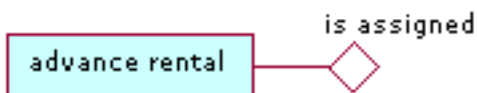
Figure H.9- Depicting the unary fact type 'advance rental is assigned' using association notation
