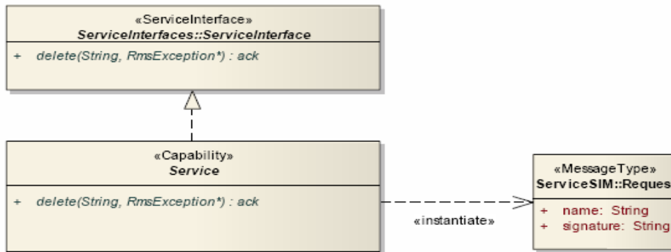
Figure 6.1 - Service Pattern Static Structure
