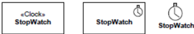
Figure 9.103 - Standard UML notation for stereotyped elements (from UML 2.5.1, Figure 12.25)
