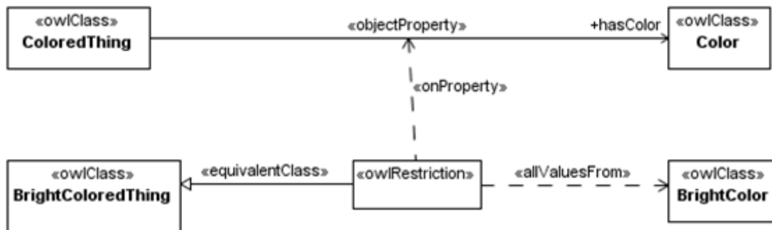
Figure 14.28 Property restriction for owl:allValuesFrom with equivalence relation using unidirectional Association notation for the property
