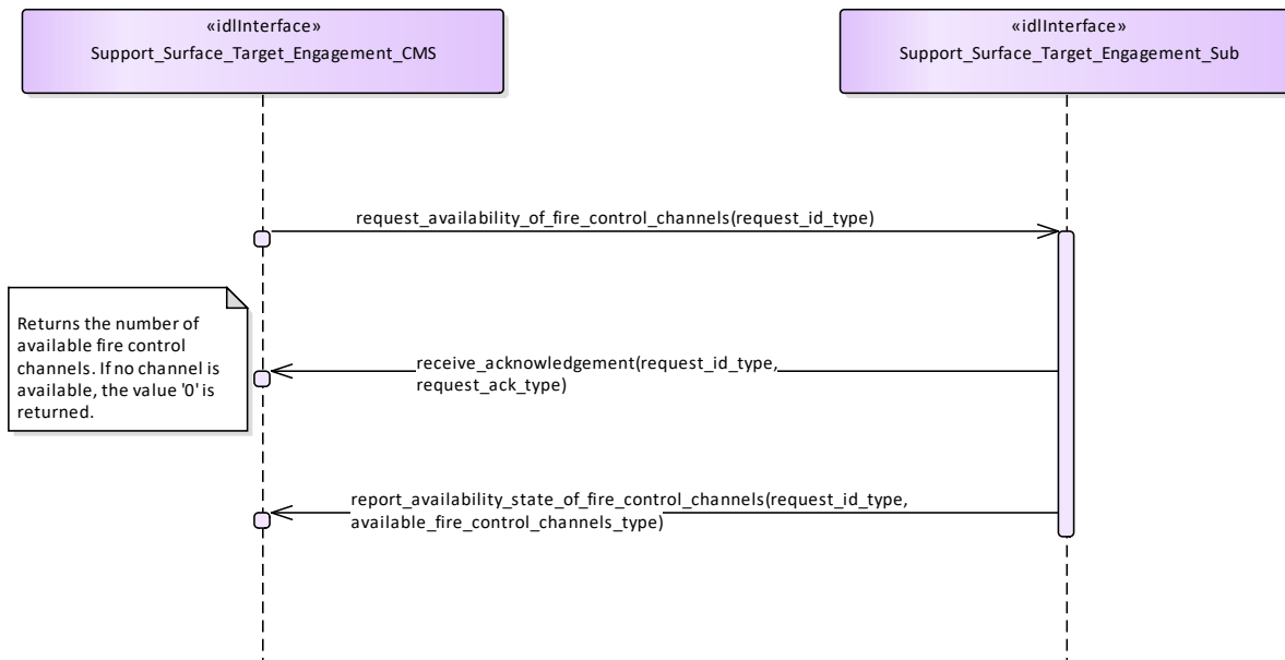
Figure 7.186 Support surface target engagement - Check availability (Interaction diagram)
