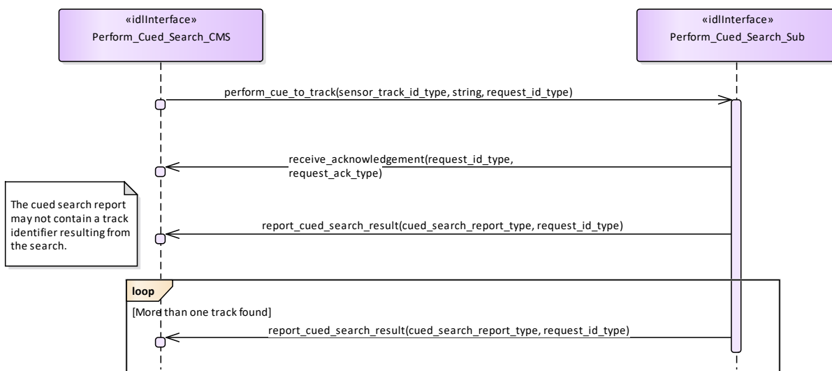
Figure 7.125 Alternative Flow - Sensor does not Perform Cued To Track (Interaction diagram)
