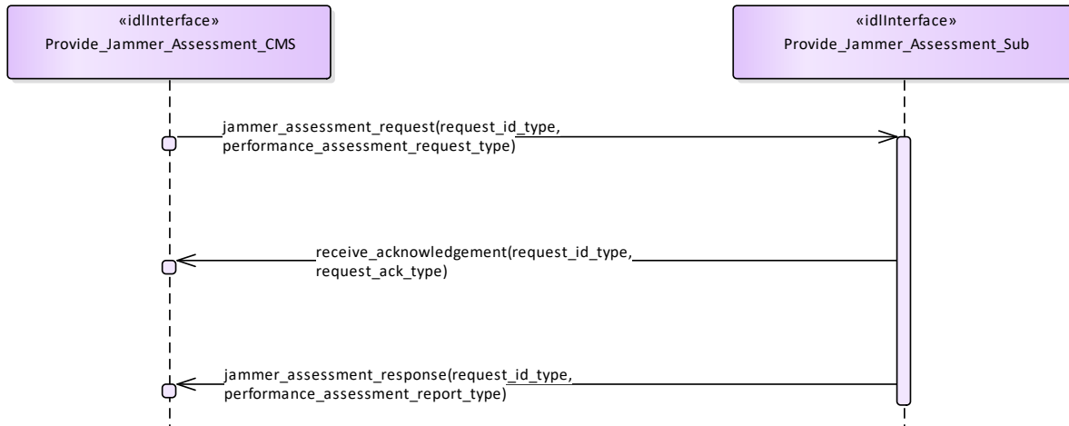
Figure 7.168 Basic Flow - Provide Jammer Assessment (Interaction diagram)
