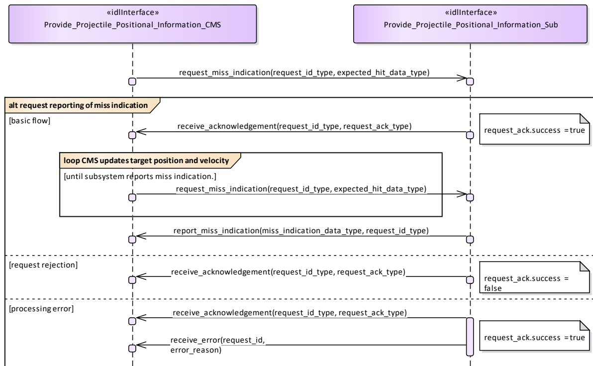
Figure 7.181 Provide projectile positional information - Request reporting of miss indications (Interaction diagram)
