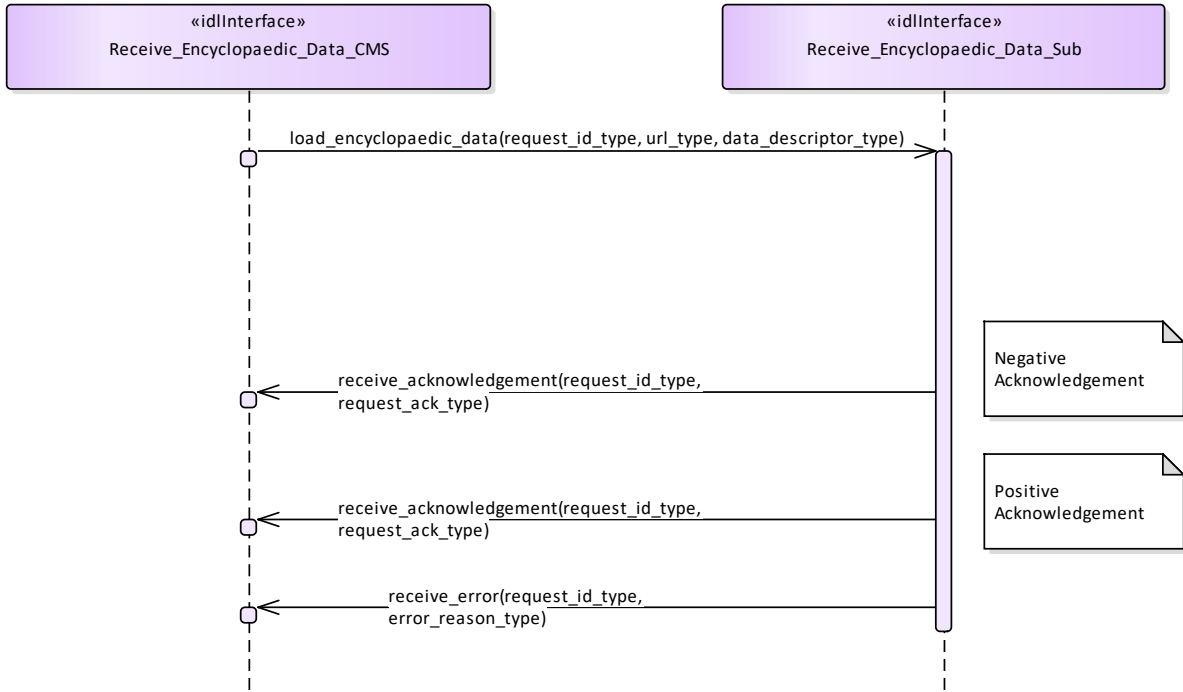
Figure 7.66 Alternate Flow - Receive Encyclopaedic Data (Interaction diagram)
