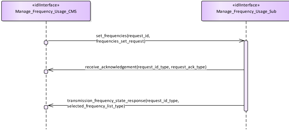
Figure 7.148 Basic Flow - Enable/Disable Frequency Usage (Interaction diagram)
