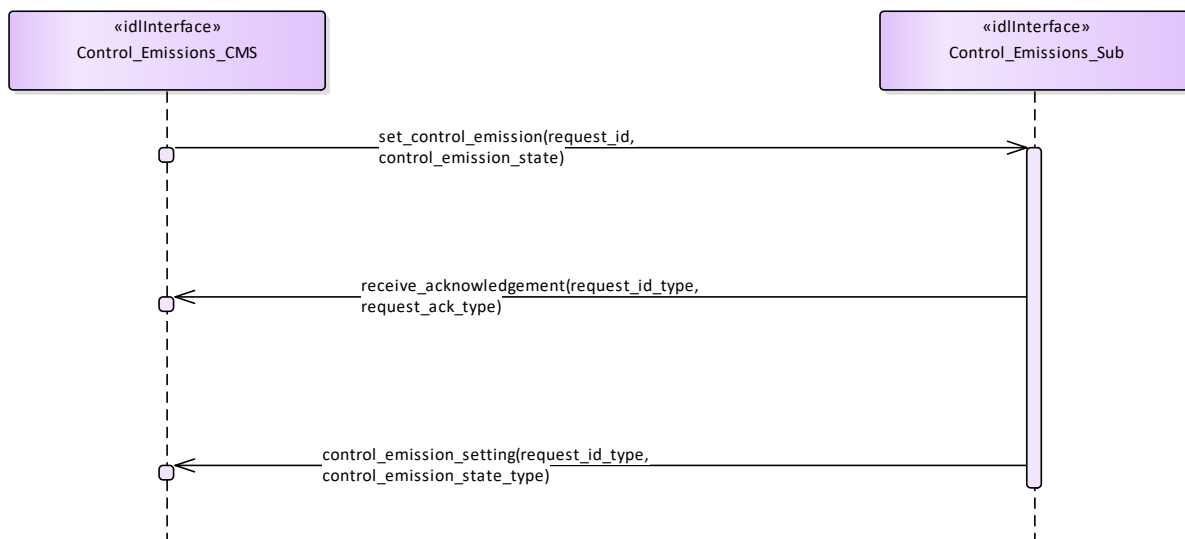
Figure 7.154 Basic Flow - Control Emissions - On/Off (Interaction diagram)
