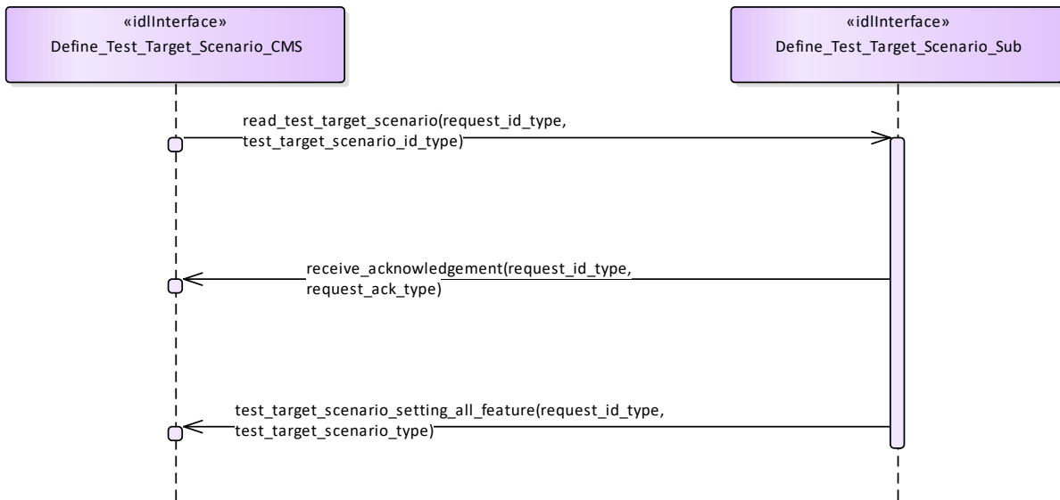
Figure 7.158 Basic Flow - Inspect a Test Target Scenario (Interaction diagram)
