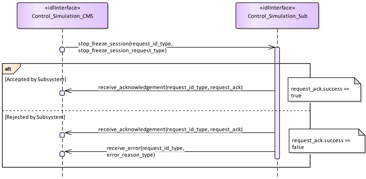
Figure 7.83 Basic Flow - Control Simulation Stop/Freeze (Interaction diagram)
