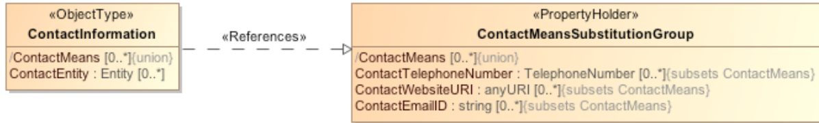
Figure 7.33 - Representation of a substitution group using UML subsetted properties in a PIM
