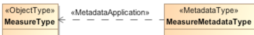
Figure 7.14 Representation of a metadata application constraint as a UML dependency in a PSM or PIM
