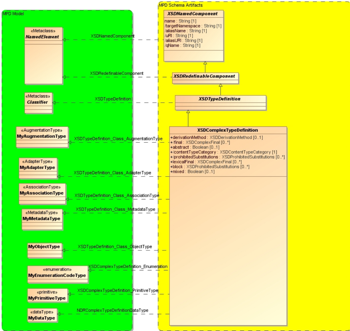
Figure 9.27 - MPD Schema Artifacts to NIEM-UML MPD Model – Type Mapping Overview
