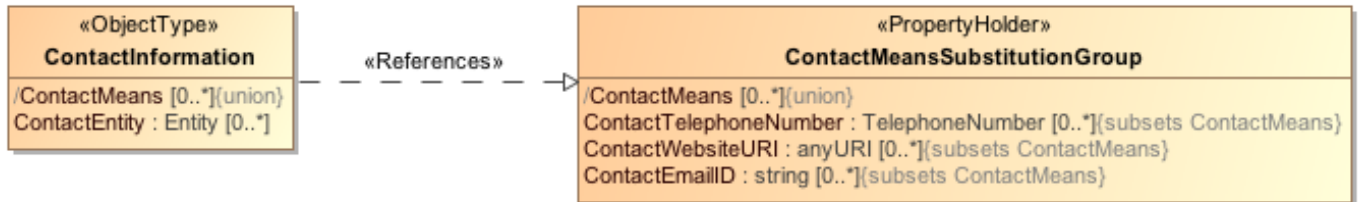
Figure 7-33 Representation of a substitution group using UML subsetting properties in a PIM
