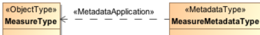
Figure 7-14 Representation of a metadata application constraint as a UML dependency in a PSM or PIM
