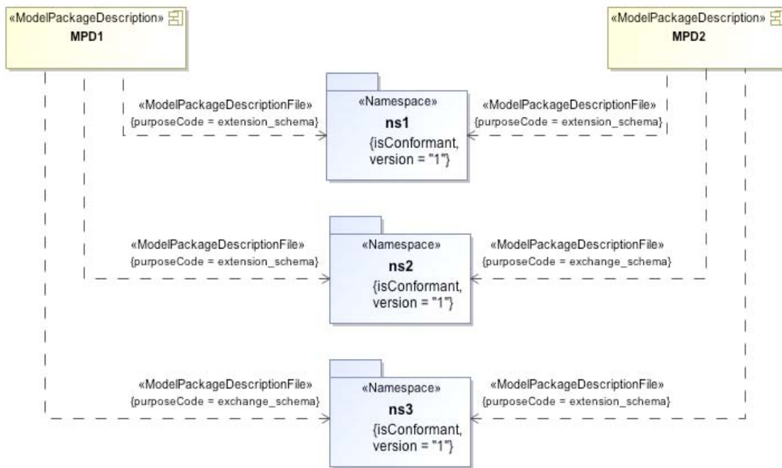
Figure 7.37 - Representation of two NIEM MPDs with included namespaces (files)
