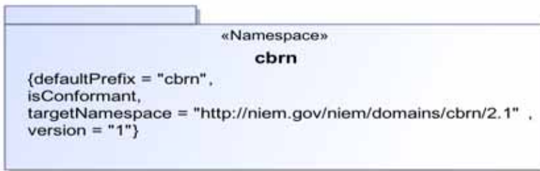
Figure 7.2 - Representation of a NIEM-conforming XML schema as a UML package
