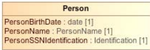
Figure 7.27 - Representation of NIEM properties as UML properties in a PIM
