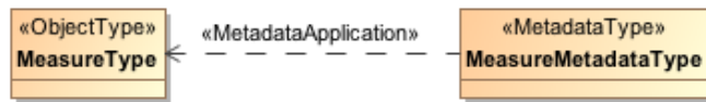
Figure 7-13 Representation of a metadata application constraint as a UML dependency in a PSM or PIM
