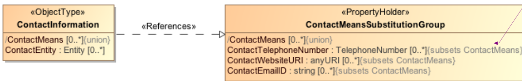
Figure 7-32 Representation of a substitution group using UML subsetted properties in a PIM
