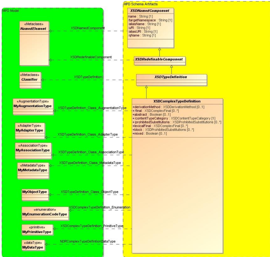
Figure 9-279-279-27 MPD Schema Artifacts to NIEM-UML MPD Model – Type Mapping Overview
