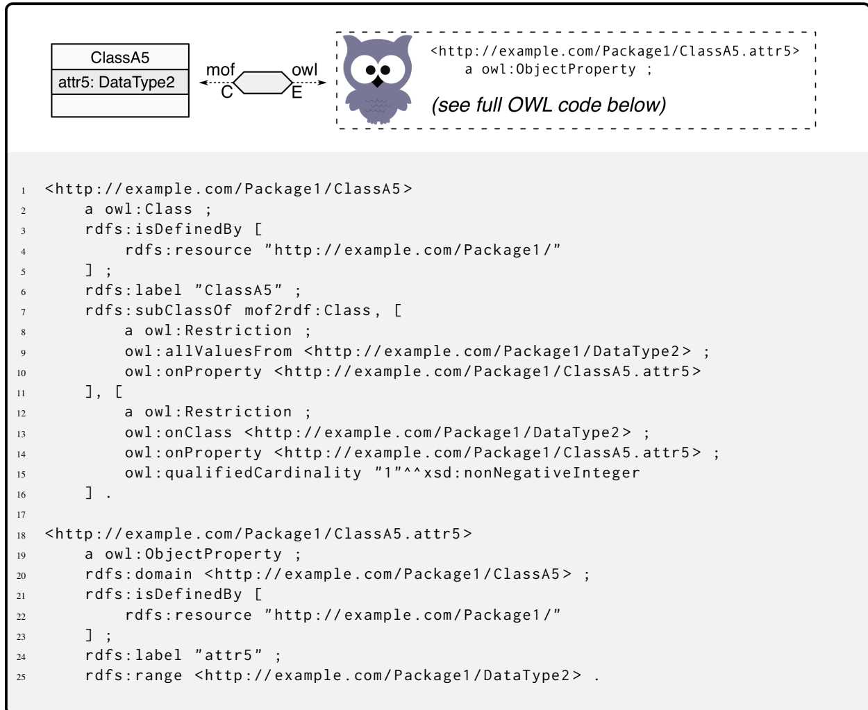
Mapping of a Property (Attribute) typed by a structured User-Defined Type, with default Multiplicity
