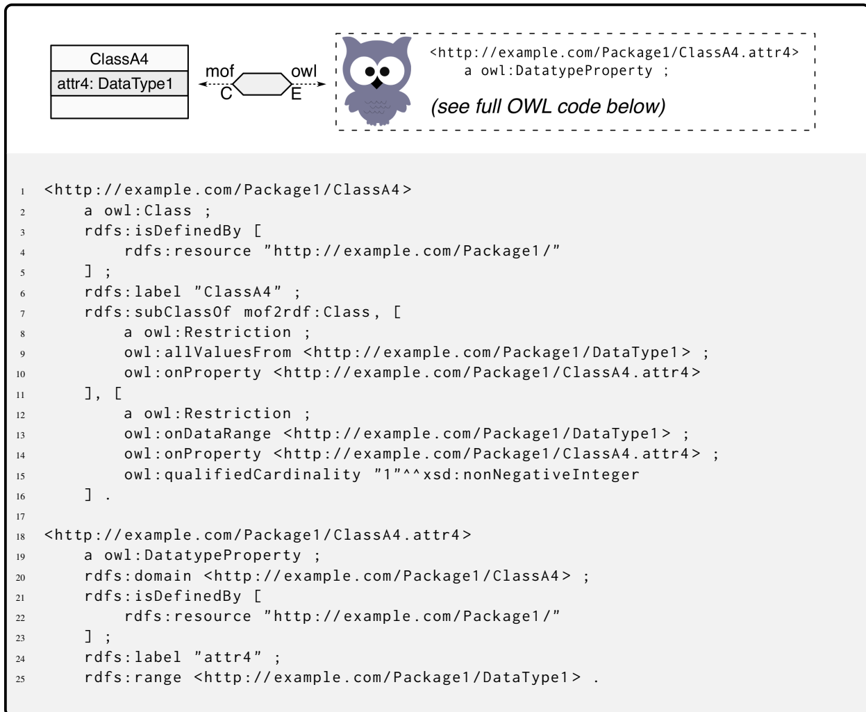
Mapping of a Property (Attribute) typed by an unstructured User-Defined Type, with default Multiplicity
