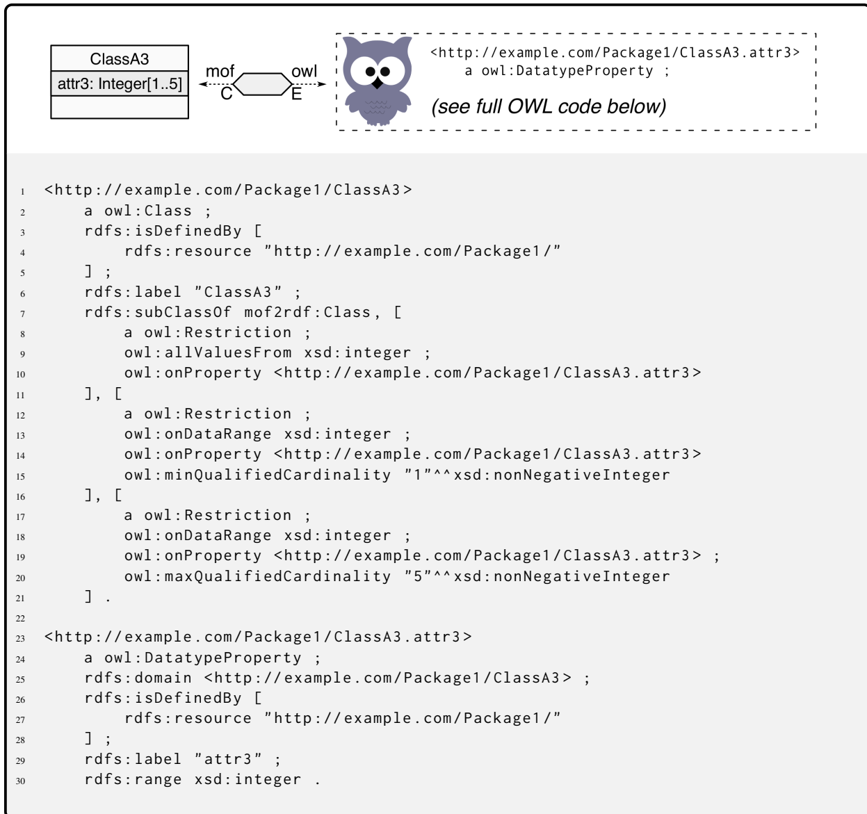
Mapping of a Property (Attribute) typed by a Literal Type, with explicit Multiplicity range
