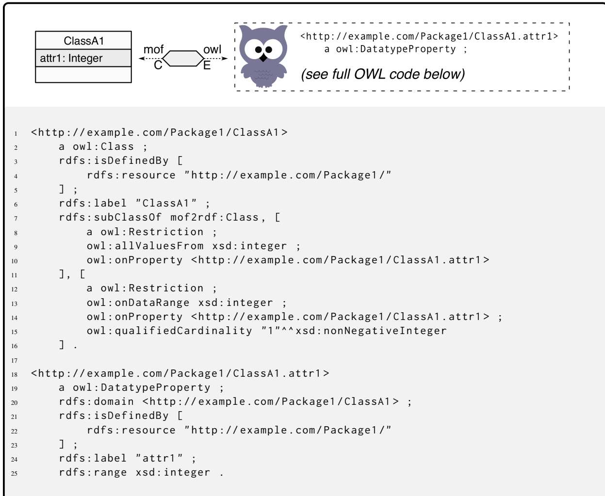
Mapping of a Property (Attribute) typed by a Literal Type, with default Multiplicity
