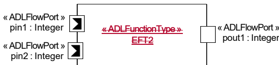
Figure A.33 - An ADL elementary function type with two input ports and one output ports
