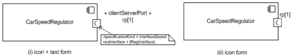
Figure 12.16 - Example of interface-based ClientServerPorts
