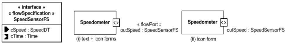
Figure 12.19 - Example of non-atomic flow port
