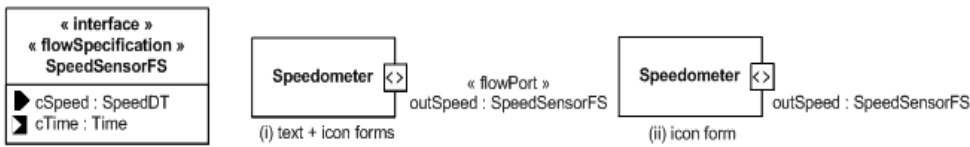
Figure 12.19 - Example of non-atomic flow port
