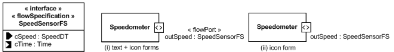
Figure 12.19 - Example of non-atomic flow port
