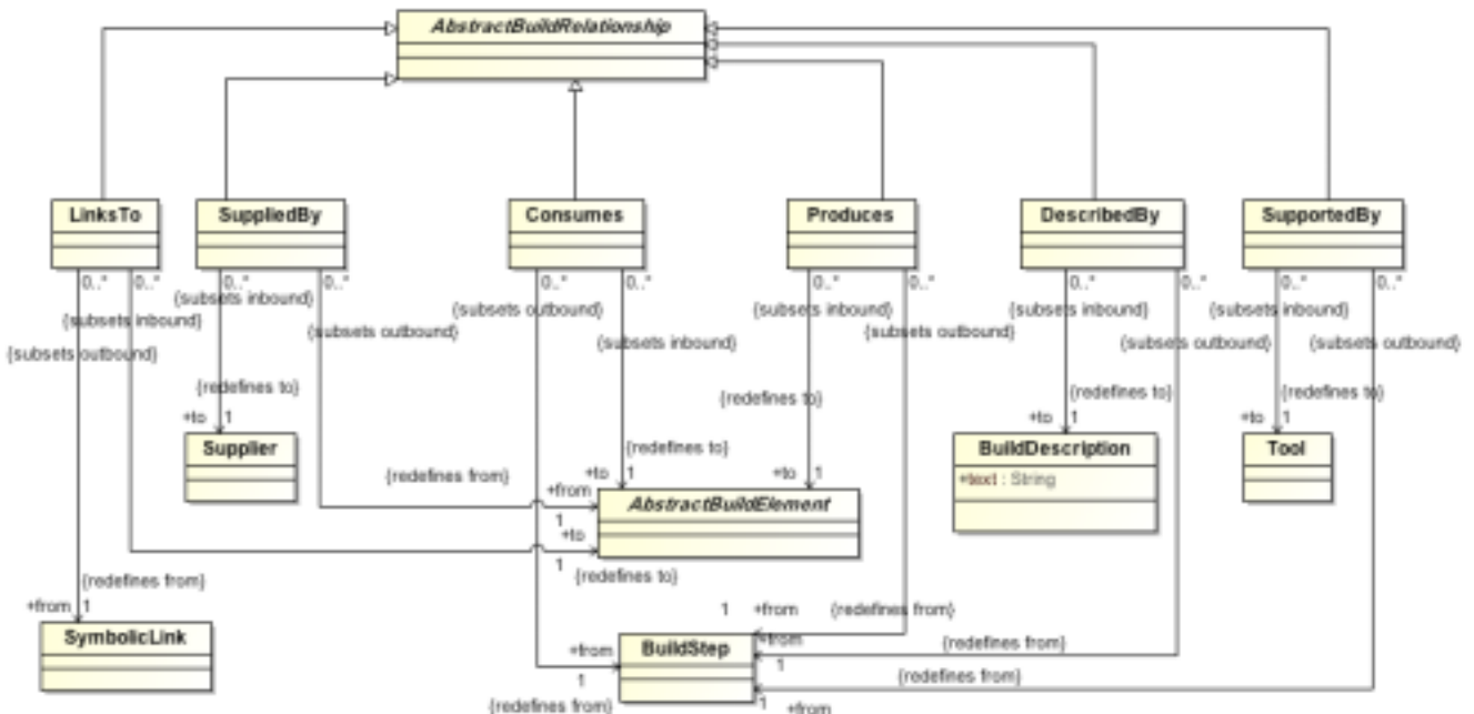
Figure 21.4 - BuildRelations Class Diagram
