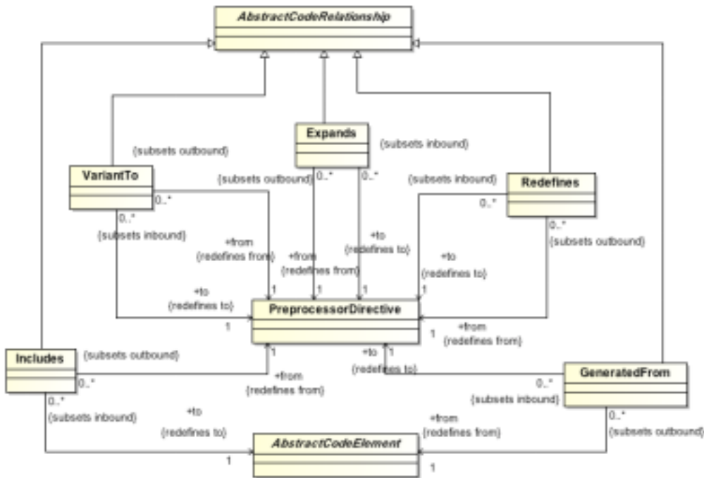
Figure 12.21 - PreprocessorRelations Class Diagram
