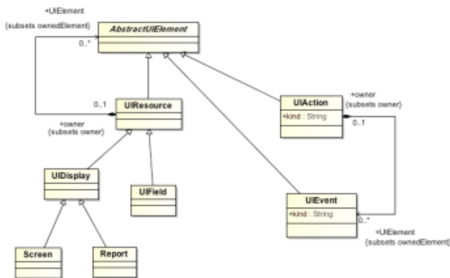
Figure 16.3 - UIResources Class Diagram
