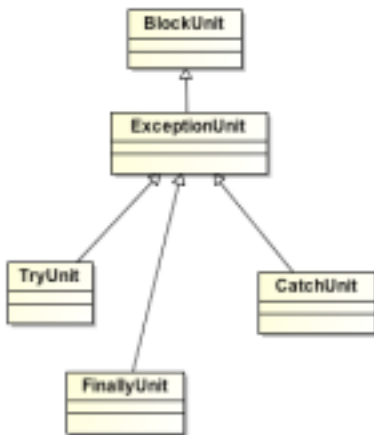
Figure 13.6 - ExceptionBlocks Class Diagram
