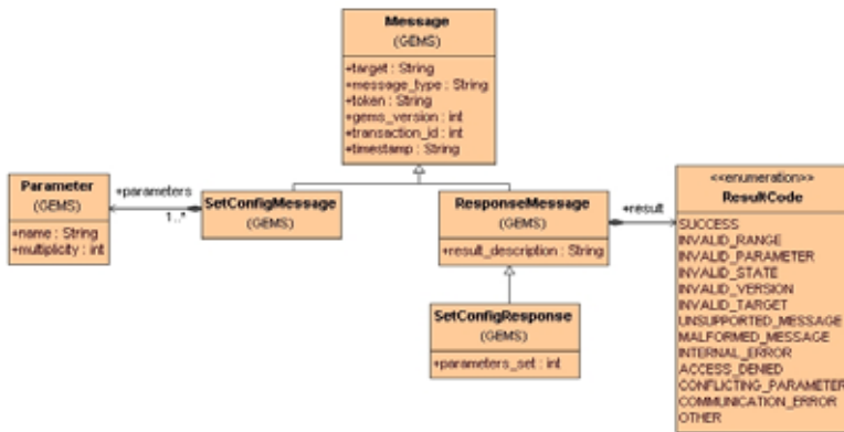
Figure 6.8 - Set Configuration Message Classes
