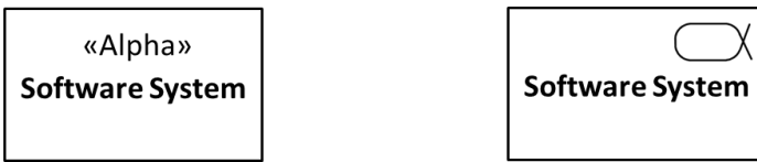
Figure 9.25 – Example visualizations of the Alpha meta-class construct and its Software System type
