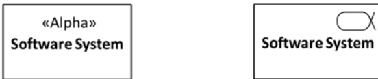
Figure 37 – Example visualizations of the Alpha meta-class construct and its Software System type
