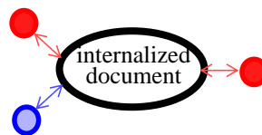
Figure 2-1 Internalizing a node returns the new object and the corresponding roles.
