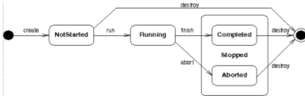
Figure 3-50 State Machine describing execution of Activities and CompoundTasks.
