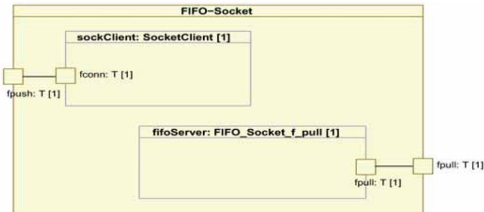
Figure 7.4 - Example of a Distributed FIFO Implementation
