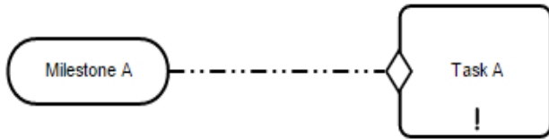
Figure 6.40 - Using the Sentry-based connector to visualize dependency between a Task and a Milestone
