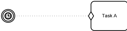
Figure 48484844: Using the Sentry-based connector to visualize dependency between a Task and a TimerEventListener
