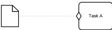
Figure 49494945: Using the Sentry-based connector to visualize dependency between a Task and a CaseFileItem
