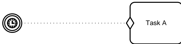
Figure 48: Using the Sentry-based connector to visualize dependency between a Task and a TimerEventListener
