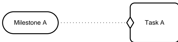
Figure 43: Using the Sentry-based connector to visualize dependency between a Task and a Milestone
