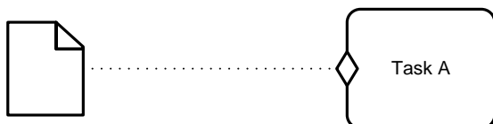
Figure 45: Using the Sentry-based connector to visualize dependency between a Task and a CaseFileItem
