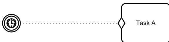
Figure 44: Using the Sentry-based connector to visualize dependency between a Task and a TimerEventListener
