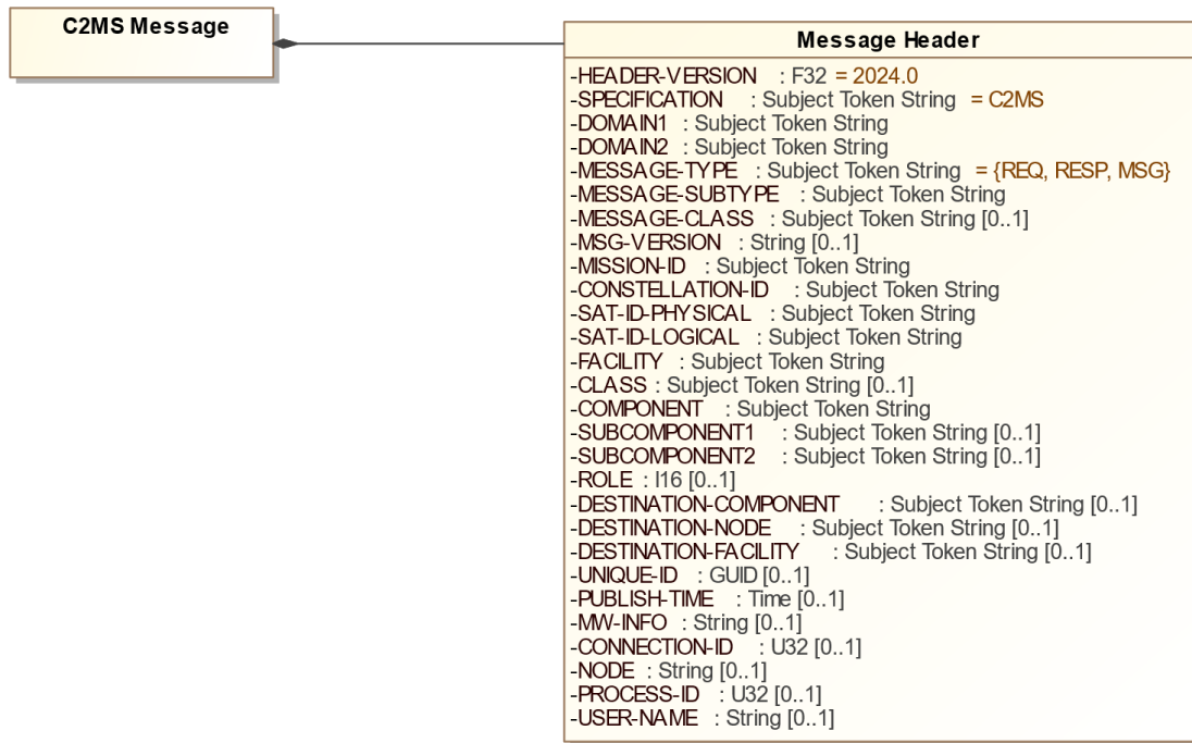
Figure 8-2. Message Header Diagram
