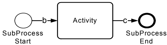
Figure 12.11 – Contents of Collapsed Sub-Process
