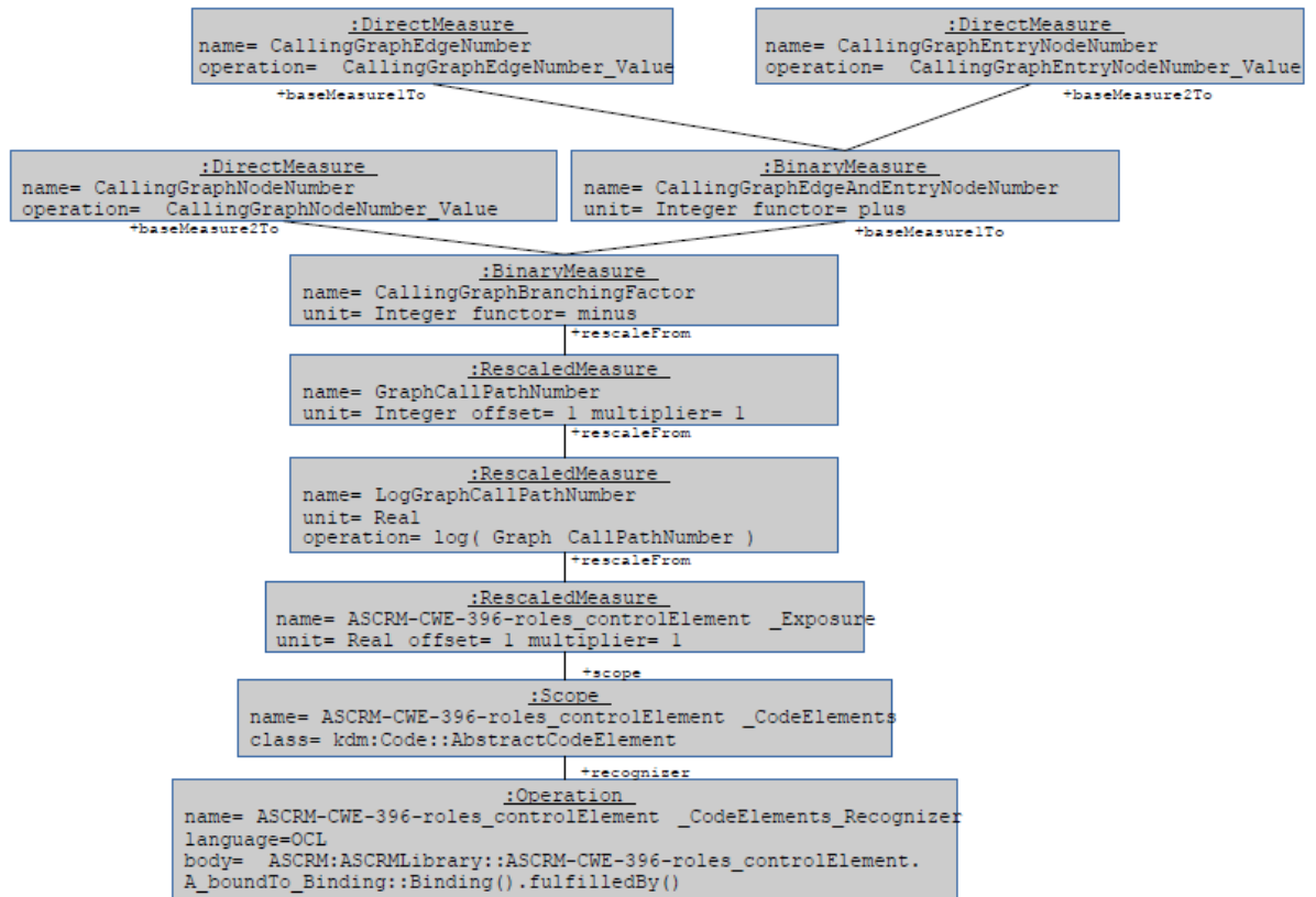
Figure 7.10 - ASCRM-CWE-396-roles-controlElement role direct exposure computation with SMM OCL Operations, Operation, DirectMeasure, Scope, and Recognizer
