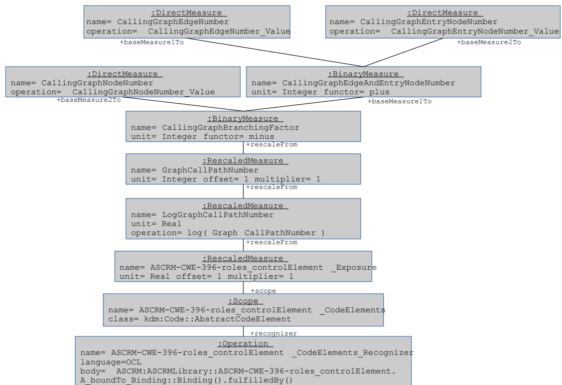
Figure 11: ASCRM-CWE-396-roles-controlElement role direct exposure computation with SMM OCLOperations, Operation, DirectMeasure, Scope, and Recognizer
