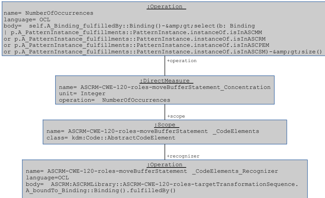
Figure 13: ASCRM-CWE-120-roles-moveBufferStatement role concentration with SMM Operation, DirectMeasure, Scope, and Recognizer
